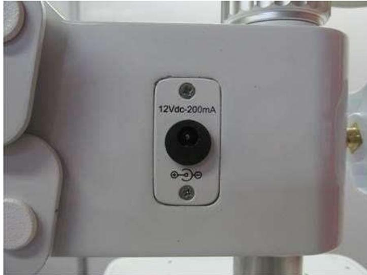
Figura 30- conector 12 V, 200 mA (CC)
